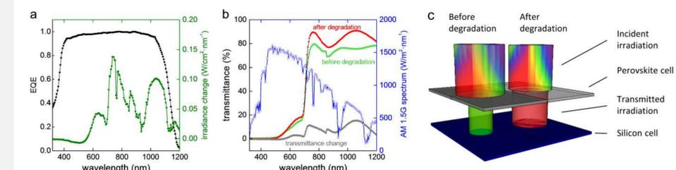
Optical degradation of the perovskite top cell may translate into  $I_{sc}$  increase at the silicon bottom cell. Based on our in-house fabricated cell, we obtained a ratio of 0.89 between the  $I_{sc}$  loss at the top cell and the  $I_{sc}$  gain at the bottom cell.
