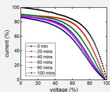
IV curves and cell parameters of an unencapsulated PSK cell are measured after various degradation times at 65 °C in air and 35% humidity.
